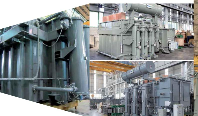
The coolers can be equipped with many accessories line: water and oil flow indicators with alarm contact, water and oil thermometers, water and oil drain taps or other special ones, on request. When water is not available, the cooling is generally OFAF.
